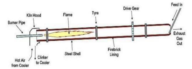
As shown in the figure below, all reactions take place in a rotating cylindrical furnace around its axis and with a gentle slope (below 5 degrees) to the ground, hematite or magnetite rocks or pellets containing coal and limestone or Dolomite enters the rotary kiln and, while moving in the opposite direction of the gas flow, heats up and regenerates at a temperature of about 1100 ° C to about 92%, and turns into sponge iron.
