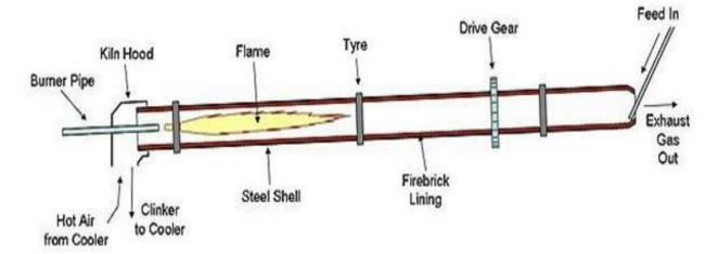
As shown in the figure below, all reactions take place in a rotating cylindrical furnace around its axis and with a gentle slope (below 5 degrees) to the ground, hematite or magnetite rocks or pellets containing coal and limestone or Dolomite enters the rotary kiln and, while moving in the opposite direction of the gas flow, heats up and regenerates at a temperature of about  $1100 \degree$  C to about 92%, and turns into sponge iron.
